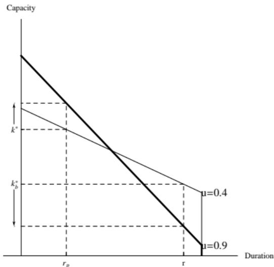
Two load duration curves and the corresponding technological mixes
